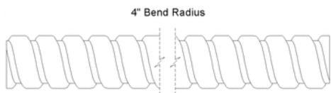
Semi-Flexible and crush proof. Available O.D. sizes 0.51" (with 4" bend radius) and larger.
