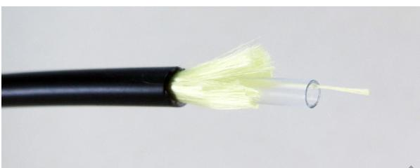
PVC over Kevlar over PTFE. Standard in the telecom industry because of the Kevlar members which prevent stretching. Ideal for small fiber sensors, D20 or RC20 and smaller. MRI compatible and liquid tight. Light crush resistance.
