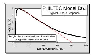
This conversion only applies when the calibration procedure has been carefully followed and the optical peak has been set at precisely 5.000 volts.
