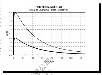
Philtec's reflectance compensated sensors were developed as the elegant solution to the problem of dynamically variable reflectance. However, using D model sensors, the problem can be solved this way. Start with test surface #1.
