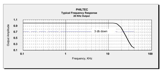
The amplitude response of a <u>standard</u> Type D sensor will have a frequency rolloff characteristic that approximates a 3 pole filter response. The chart above shows that typical response. With the 3 db down point set at 20 KHz, the output is flat out to approximately 15 KHz.
