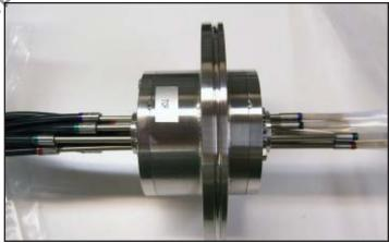
\* Inside the BvF, a Ø 25 mm fused fiberoptic image rod passes the sensor signal channels across the vacuum bulkhead. The glass rod is sealed with a Swagelok™ Ultra-torr compression fitting which is welded to the I.D. of the BvF. Precision machined end caps contain 16 ports on each end for accurate alignment of the fiberoptic bundles.
